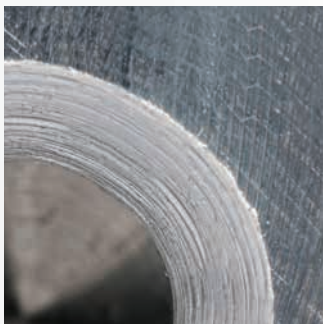
Countersinking with standard countersink
